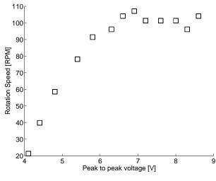
Figure 11: RPM for a rotor driven at 7.6 MHz.
