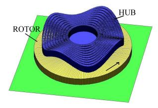
Figure 4: Hub resonance actuating the rotor
