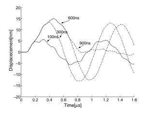
Figure 3: Simulated silicon surface displacement for different pulse widths
