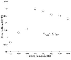
Figure 9: Rotation speed for a pulsed rotor
