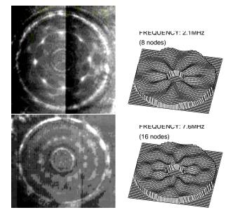
Figure 12: Interferometric image of resonant actuated rotor in vacuum showing nodes and corresponding simulated mode of the hub.
