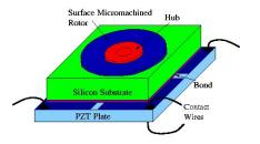
Figure 2: Surface micromachined rotor actuated with PZT plate
