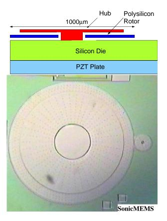
Figure 5: Polysilicon rotor fabricated using SUMMiT process
