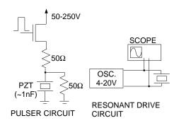
Figure 6: Driving circuits used for actuation
