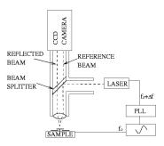
Figure 7: Interferometer and high speed camera set-up
