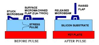
Figure 1: Surface micromachine actuation using stress pulses [8, 9]
