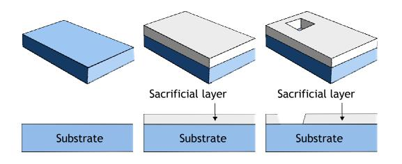
Semi-3D structures are made, by repeating the steps of film deposition and film patterning.
