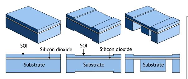
Thick structures are made of etching the entire silicon wafer. Device is encapsulate with wafer bonding.
