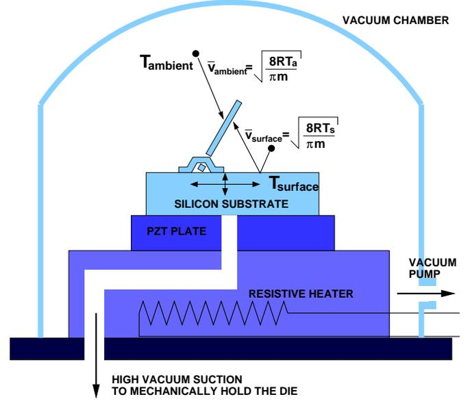
**Figure 1.** The origin of thermo-kinetic force. Gas molecules leaving the heated surface have higher momentum than those in the ambient gas. Also shown is the experimental set-up and the assembly jig. The two vacuum ports are for maintaining differential pressure over the die for hold down suction.
