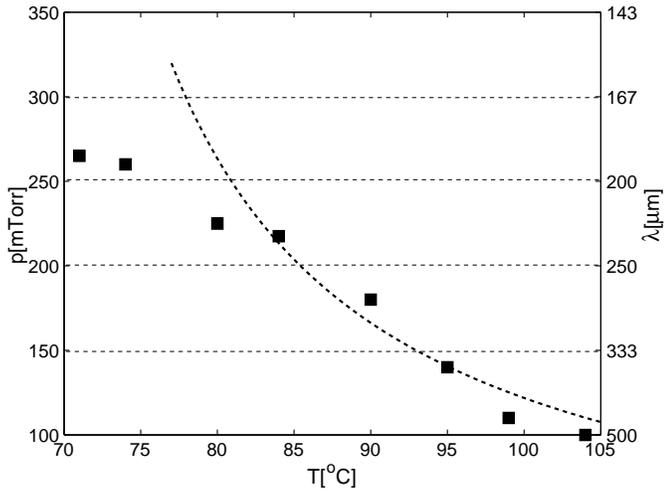
**Figure 4.** Measured flap falling pressure thresholds versus substrate temperature and the theoretical  $p$ - $T$  curve ( $\alpha = 0.8$ ). Right y-axis shows the calculated mean free path at 25°C (flap length 400  $\mu\text{m}$ ).
