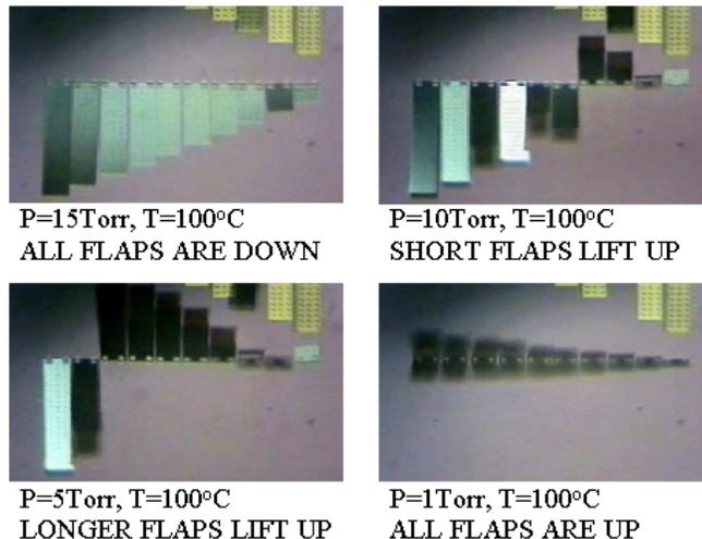
**Figure 3.** The effect of flap length on the transition pressure from viscous to molecular flow. As the chamber pressure is lowered, shorter flaps are lifted before longer ones.
