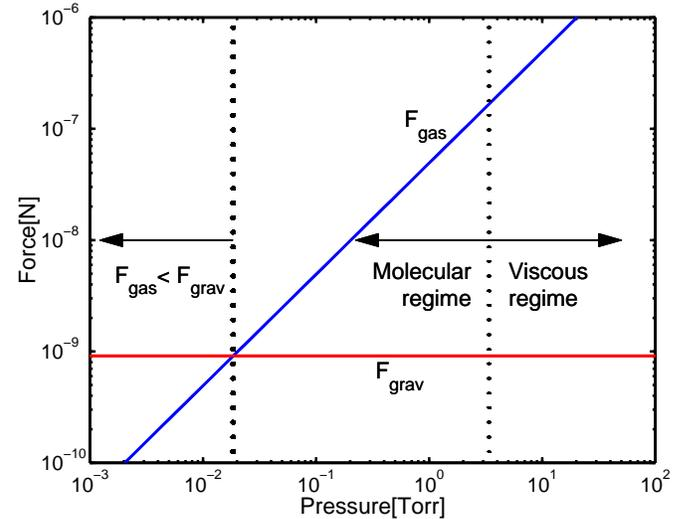
**Figure 2.** Thermo-kinetic force  $F_{gas}$  and gravity force  $F_{grav}$ . Above  $\sim 10$  Torr (viscous regime), there is no net force on the flaps. Below  $\sim 10$  Torr (molecular regime), the flaps feel net force upwards. The gravity force dominates below  $\sim 10$  mTorr.
