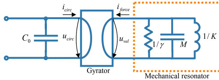
**Figure 4.** Voltage analogue for a mechanical resonator ( $v = u_{vel}$  and  $f = i_{force}$ ).
