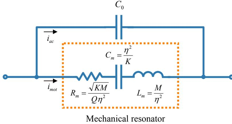
**Figure 2.** Electrical equivalent circuit for microresonator.
