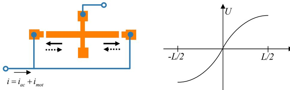
**Figure 1.** Schematic of longitudinal mode beam resonator and the vibrational displacement (mode shape) [1].
