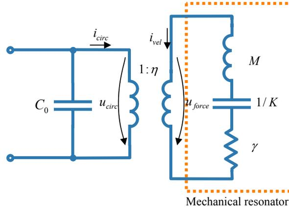
**Figure 3.** Current analogue for a mechanical resonator ( $v = i_{vel}$  and  $f = u_{force}$ ).
