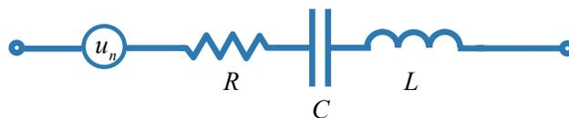
**Figure 1.** RLC resonator with noise generator  $v_n$
