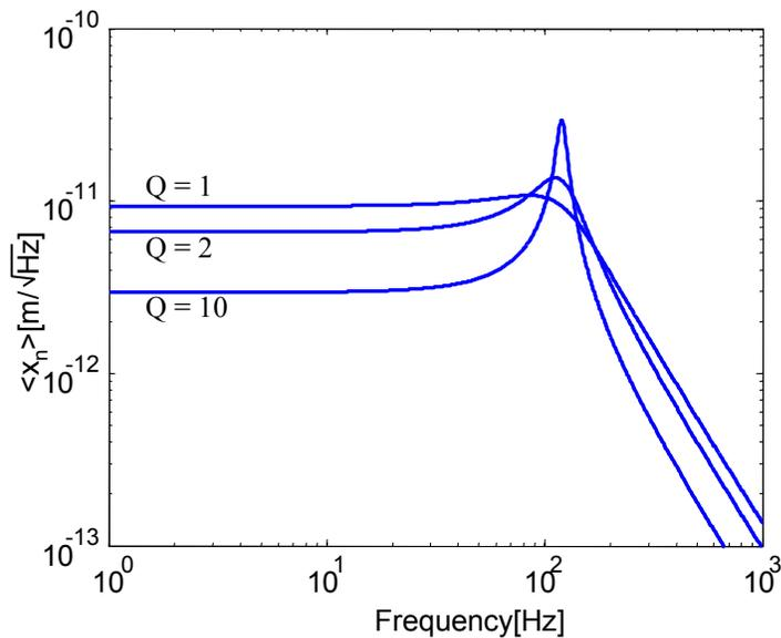
**Figure 4.** The calculated accelerometer noise spectrum.
