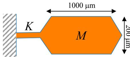
**Figure 3.** A schematic of MEMS accelerometer.
