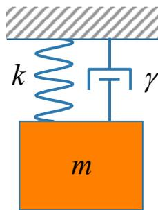
**Figure 2.** Mechanical resonator represented with mass  $M$ , spring  $K$ , and dash pot damper  $\gamma$ .
